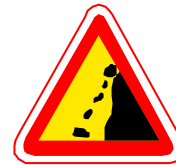
Falling rocks. Indicates stretches of road where there is danger of falling rocks.
