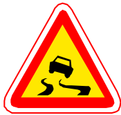
Slippery road. Indicates stretches of road that may be slippery when wet or dirty.
