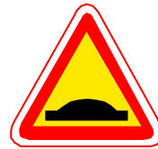
Speed bump ahead. Indicates a speed control device (speed-bump/hump) is ahead.
